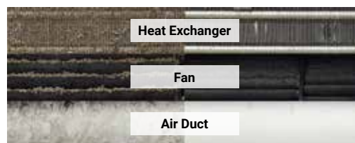
Without Dual Barrier Coating (After 10 Years)
